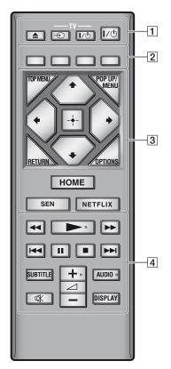
$\checkmark$ ,  $\square$  +, and AUDIO buttons have a tactile dot. Use the tactile dot as a reference when operating the player.
